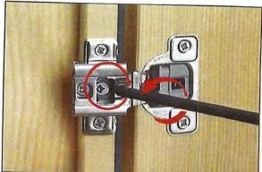
Side adjustment by eccentric cam for hinges: CU\_37D\_R - CU\_34D\_R = **+2.5mm (3/32") / -1.8mm (1/16")**CU\_32D\_R - CU\_3AD\_R - CU\_3CD\_R = **+3mm (1/8") / -2mm (3/32")**
